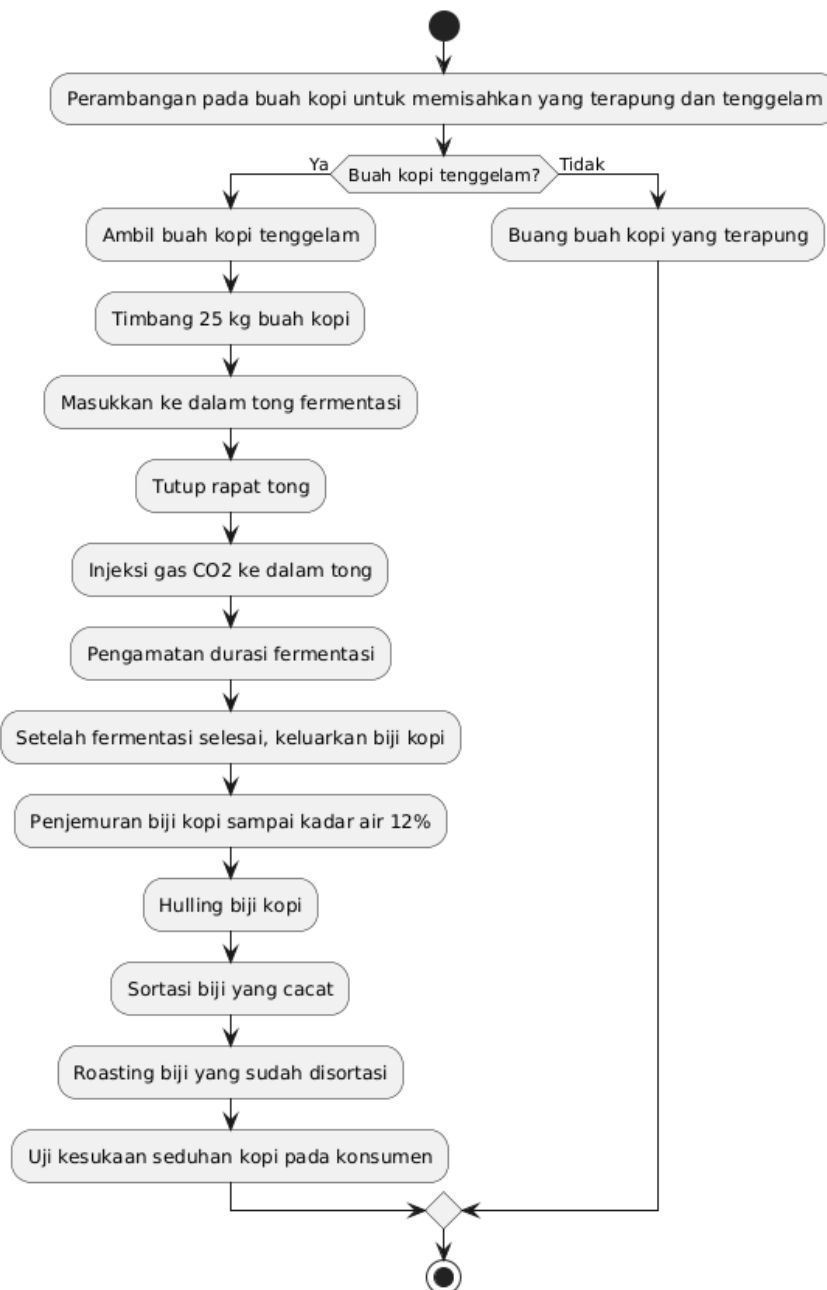
Figure 1. Steps of the Carbonic Maceration Method
