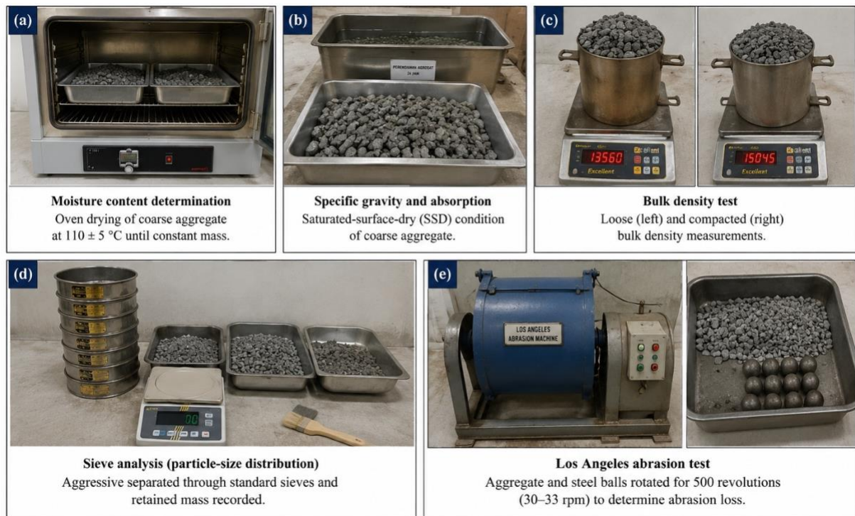
Figure 2. Material characterization procedures: (a) oven drying for moisture-content determination; (b) saturated-surface-dry aggregate preparation; (c) bulk-density measurement; (d) sieve analysis; and (e) Los Angeles abrasion testing.
