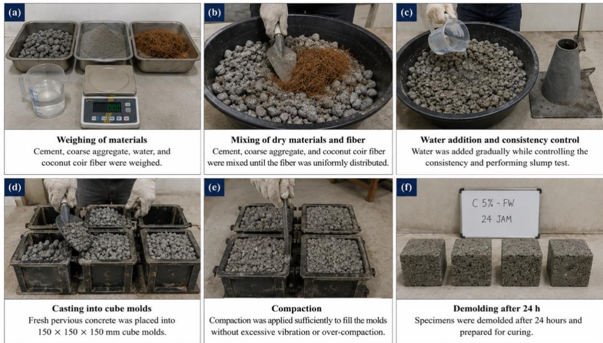
Figure 3. Preparation of coconut coir fiber-reinforced pervious concrete: (a) weighing constituent materials; (b) mixing cement, coarse aggregate, and coconut coir fiber; (c) controlling fresh-mixture consistency; (d) casting into cube molds; (e) compaction; and (f) demolding after 24 h.
