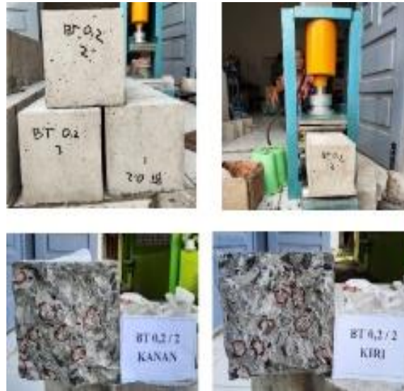
Figure 5. Fiber distribution in concrete beams
